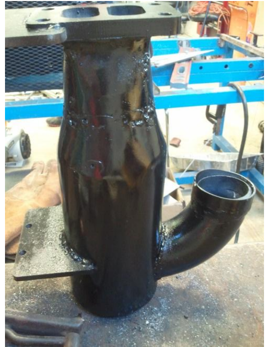
Figure 30: Combustor. The combustor is where the air and the fuel are mixed and heated to produce the energy to move turbine.
