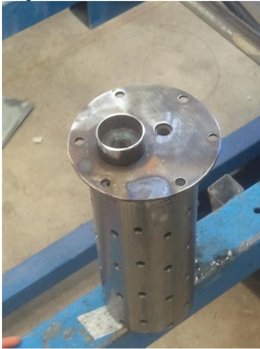
Figure 29: Combustion Liner. The combustion liner function is to obtain a more uniform air flow inside the combustion chamber.
