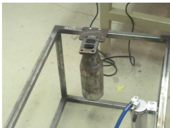
Figure 17: The combustor mounted to the frame using a \frac{1}{2} thick plate and two screws.
