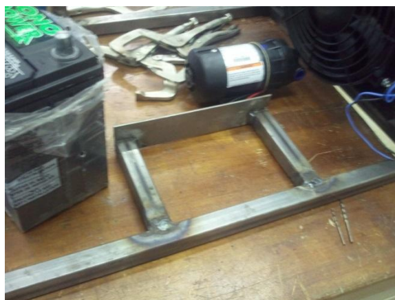
Figure 16: Battery support built with two square tubes and a plate.
