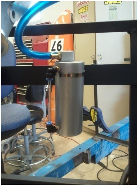
Figure 33: Oil Can. The oil can is used to store the lubricator (oil).
