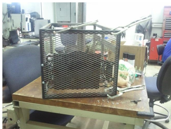
Figure 12: Assembly of the oil cooler and safety screen.
