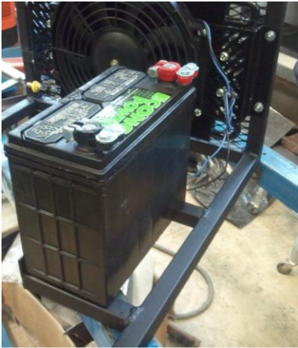
Figure 37: 12V Battery. The battery is the source of energy to power the electrical equipment of the gas turbine.
