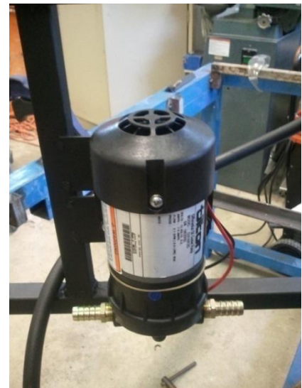
Figure 32: Oil Pump. The oil pump is responsible of distributing the lubrication (oil) along the system.
