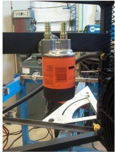
Figure 34: Filter Mount. The filter is used to filter the lubricator of little particles so other part won't be affected.
