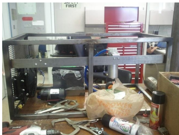
Figure 13: Oil filter and oil catch can positioned with screw to the rectangular plate
