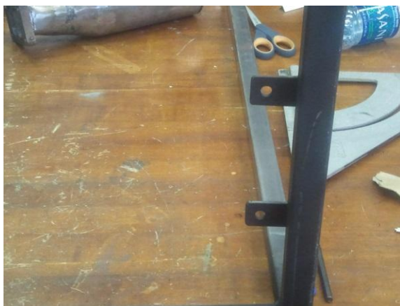
Figure 5: Two plates of 2 "L x 1" W x 1/8" thicknesses welded to the frame to mount the oil cooler.
