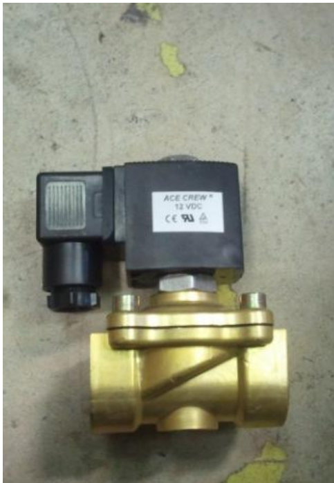
Figure 35: Solenoid. The solenoid is responsible to cut the gas flow if the gas turbine needed to be shutdown.
