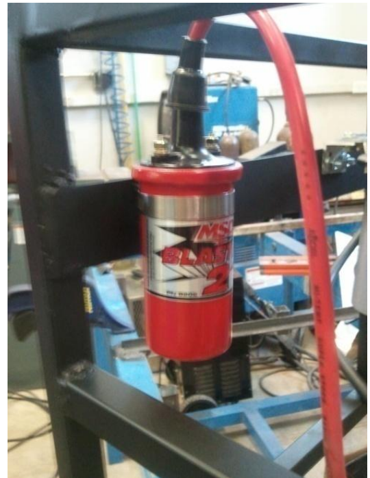
Figure 36: Ignition Coil. The ignition coil is responsible to send the required voltage to create the spark in the ignition.
