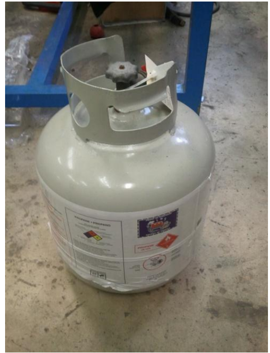
Figure 38: Gas Cylinder. The gas cylinder is the source of fuel for the system.
