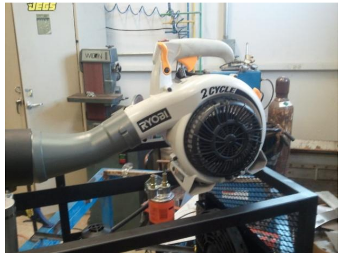
Figure 40: Gas Blower-Vac. The Blower is used to start up the system.
