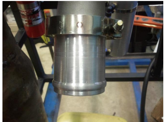
Figure 44: Turbo Pipe. The turbo pipe is used to connect the air hose to the turbocharger.
