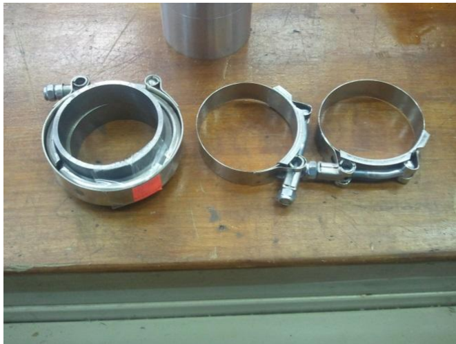
Figure 43: V-clamps. The V-clamps are used to secure hoses and pipes.
