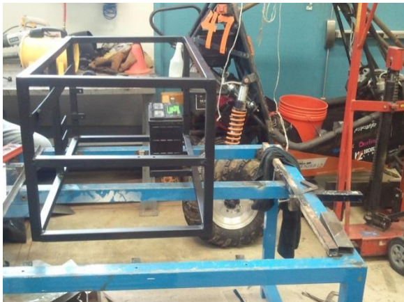
Figure 21: A square tube was added to the frame to support the weight of the combustor and turbine
