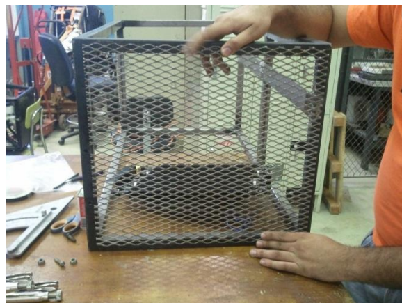
Figure 8: Installation of a fence to one side of the frame to protect the oil cooler
