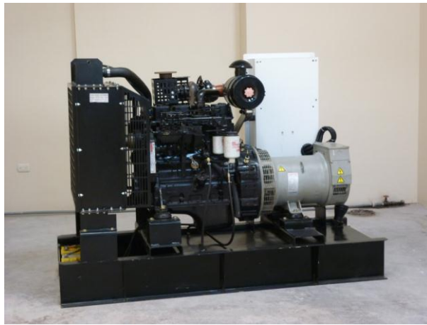
Figure 2: Diesel Cycle Generator Set
