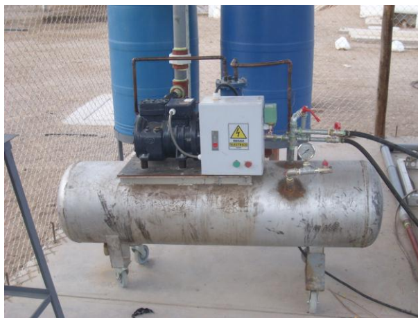
Figure 4: H 2 S Removal (back) and Compression System (front)
