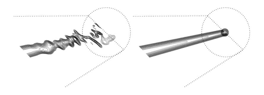
Injecting dye as Reynolds did Flow time developing Dye space evolving
